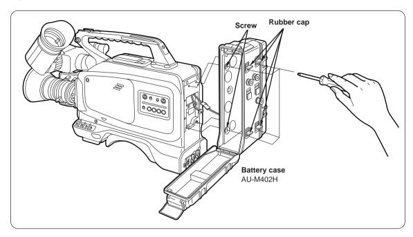
Holes with the screws recessed inside can be seen when the cover is opened and the rubber caps are lifted. Tighten up these screws using a screwdriver so that the battery case is mounted onto the unit. Tighten the screws up all the way.
